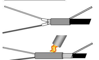
J. Center the 3" length of heat shrink tubing over the connection. Apply heat evenly to shrink tubing around the heating cable, barrel connectors and power leads. Do not burn the heat shrink.
