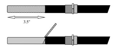
D. Pick the braid apart near the outer jacket and pull the cable through the opening in the braid. Twist the braid into a pigtail.
