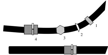
B. Assemble the connector and tighten, leaving six inches of cable extending through the connector.
