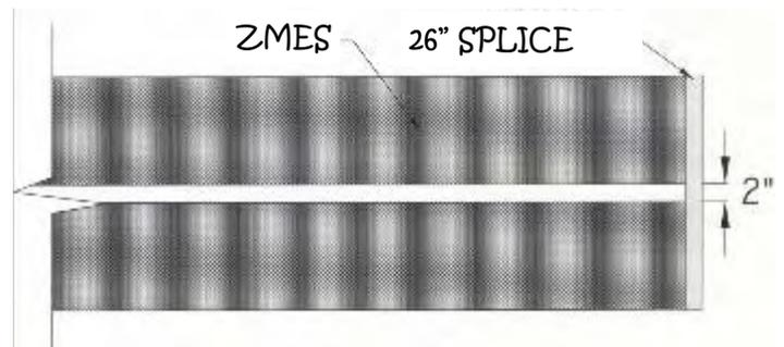
**ZMesh Cut Repair.** Always use a ZMesh Cut Out Kit whenever the ZMesh has been cut or damaged, or whenever a portion of the ZMesh must be cut away to avoid an object. Never cut away more than 4" of 12" ZMesh nor more than 3" of 9" ZMesh. Use Heatizon Systems ZMesh Cut Out Kit (Heatizon Part # CUTOUTKIT).
