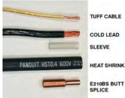
**Step 2: Crimp connection.** Slide the heat shrink tubing and sleeve over the Tuff Cable to a point at least 8" beyond the splice. Insert the Tuff Cable and the Cold Lead into the E210BS butt splice connector. Crimp the connection in two locations on each side of the lug.
