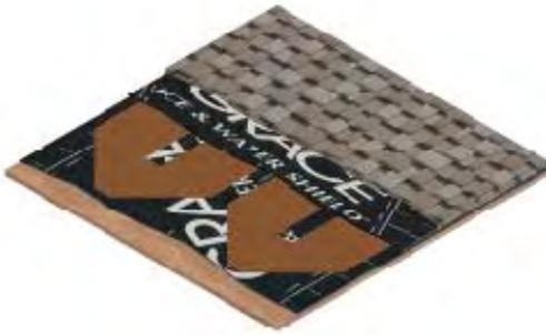
ZMesh Heating Element can be used for de-icing in valleys and on eaves as well as other trouble areas on roofs. The ZMesh must be covered with Ice and Water Shield (Part Number NI114) or EPDM (Part Number NI133). These products may also be used under the ZMesh element if desired. Great care must be taken to make sure that the element is shielded from moisture. Al-
