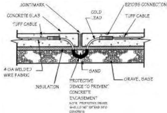
*Tuff Cable heating element can be jumpered by using a Heatizon Jumper Kit. All jumpering of element is to be done using Heatizon Cold Lead (E210) only. All Butt Splices (E210BS) must be imbedded in a heat sink.*
