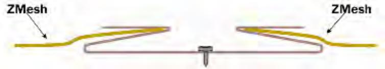
**Jumper Plate.** When two adjacent areas are being jumpered together, or connected in series, a Wall Plate or Jumper Plate (Heatizon Part # E219) is used to extend the ZMesh through a 2" x 4" wood studded wall, by installing the jumper over a wood 2" x 4" footer stud. Follow the instructions in Section 7, "Making the Connection."
