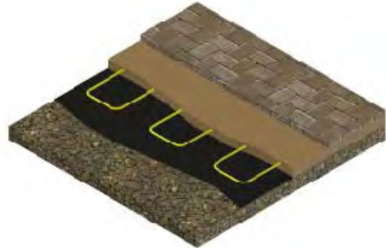
**Step 1.** Cover entire area to be heated with rigid 1" thick insulation, and then 1/2" of sand.
