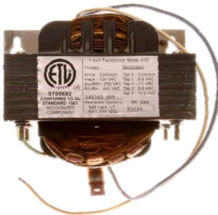
All single Heatizon Systems Transformers require one pair of Cold Leads (SLC 500 systems require one pair of Cold Leads for the beginning and ending points of the Tuff Cable or ZMesh heating element). One of the Cold Leads from any given pair connect to the common tap located at the back of the Transformer and the other Cold Lead connects to one of the voltage taps at the front of the transformer.
