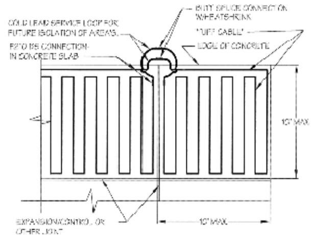
See Section 7, "Making the Connections" for more details on how to make this connection..
