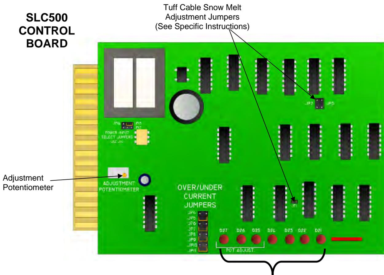
**NOTE:** LED's are designated as D21 through D27 (under current indication is D21, D23 is Transformer Overtemp, D24 indicates the activator is not calling for heat and D25-D27 indicate proper potentiometer adjustment). Also a status indicator is located on the front cover door of the SLC500 Control Unit. This indicator mimics the function of the status indicator LED on the activation device.
