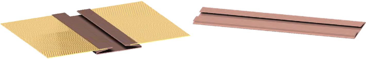
Step 1: Cut both runs of ZMesh to be spliced, leaving the cut straight and flat. Remove any loose strands. Insert first section of ZMesh into one side of the Z splice plate. Gently crimp or compress Z fold; ensure that ZMesh stays fully inserted in the fold. Repeat this procedure with second length of ZMesh.
