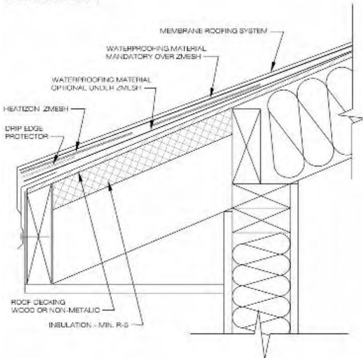
Eave Detail — ZMesh Under Single Ply Membrane
