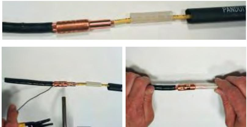
**Step 4: Heat shrink connection.** When the splice has completely cooled slide the heat shrink and center it over the splice. Use a broad soft flame torch or hot air gun to heat around the diameter of the tube to warm and shrink it. Do not scorch the tube. The shrink is complete when adhesive oozes from between the tube and the Tuff Cable and Cold Lead.
