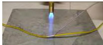
**Step 5. Secure the repaired Tuff Cable in place.**
