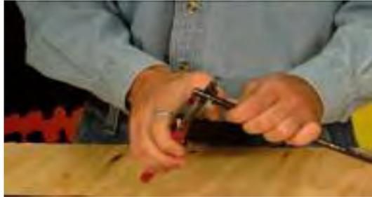
**Step 2: Crimp connection.** Slide the heat shrink tubing and sleeve over one Cold Lead to a point at least 8" beyond the splice. Insert the Cold Leads into the E211 butt splice connector. Crimp the connection in two locations on each side of the lug.
