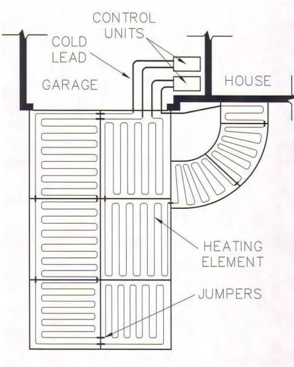
Sample Driveway and sidewalk layout for two zones of Tuff Cable snow melting systems. Note that jumpers extend the Tuff Cable heating element through all joints and marks.
