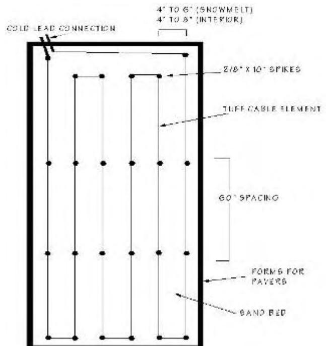
Sample Layout of Tuff Cable Under Pavers
